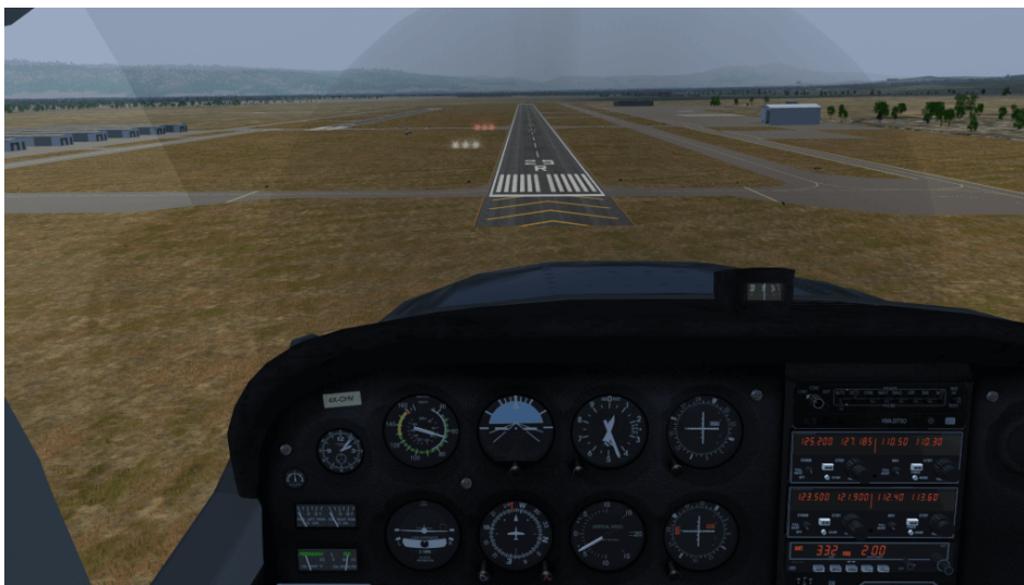
Figura 9.18: On Final at Livermore with VASI on the left
