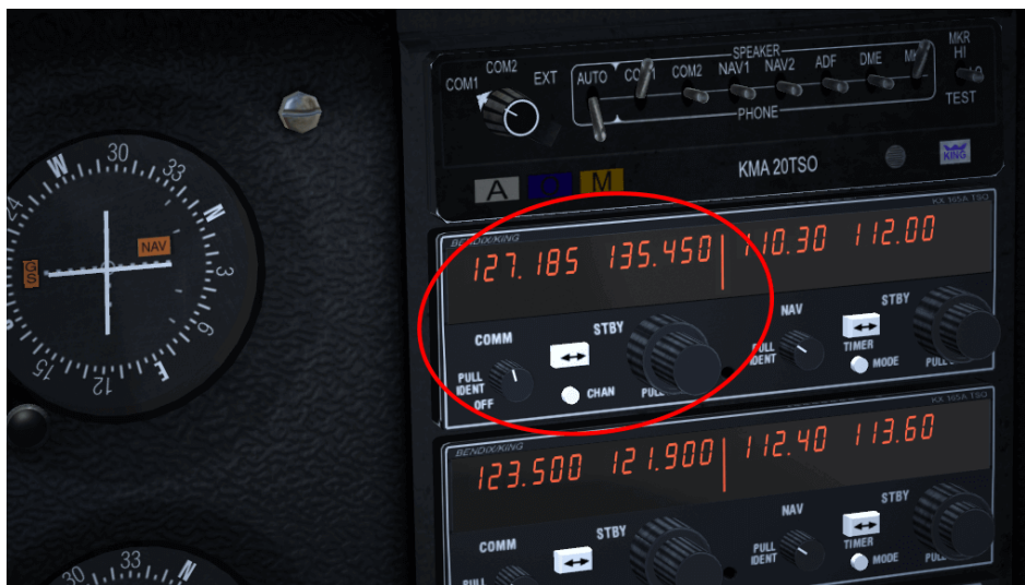
FIGURE 9.4 – The C172 communications stack with COMM1 highlighted
