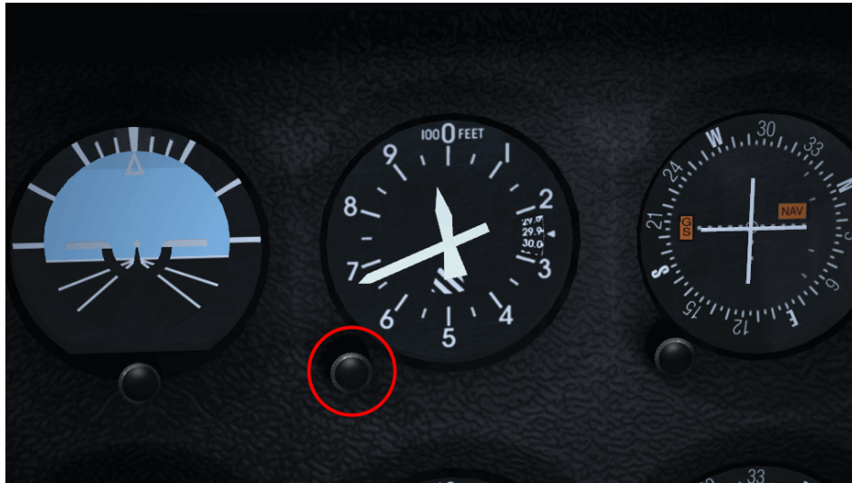
FIGURE 9.8 – Altimeter calibration knob
